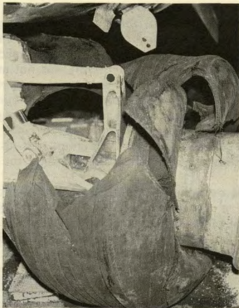
Tire and wheel assembly with blowout plug still intact.
